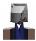
Internal coolant is recommended for optimum chip flow and tool life.
